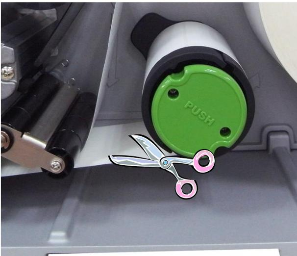
1. Break the liner between peel-off roller and the internal rewind spindle.
