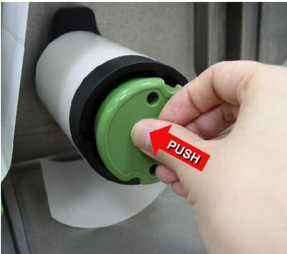
2. Push the liner release button to release the liner on the internal rewind spindle.
