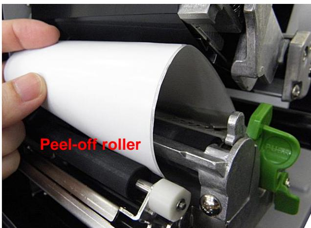
6. Feed the label between peel-off roller and platen roller.
