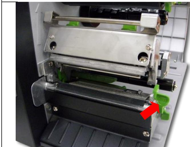
2. Push the print head release lever to open the print head mechanism.
