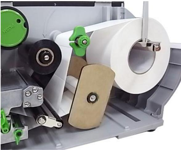
4. Insert another supply holder guide into the internal rewind for 1" core label roll.
