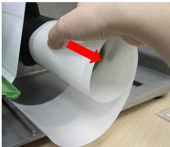
3. Slide off the liner from internal rewind spindle.
