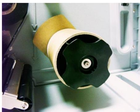
1. Insert media into the printer label spindle. Pull label roll leading edge forward through the media guide bar, damper media sensor and place the label leading edge onto the platen roller.
